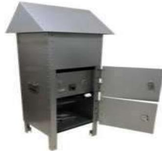
Gambar 2. *High Volume Air Sampler (HVAS)*
