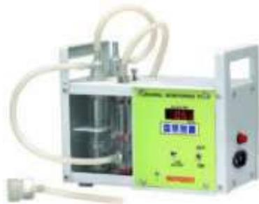
Gambar 3. *Low Volume Dust Sampler (LVDS)*
